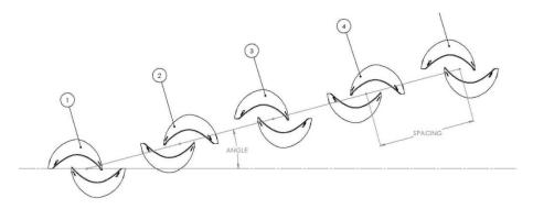
The same distances and angles would work in an arrangement of two rows. This is an alternative that also works well:
